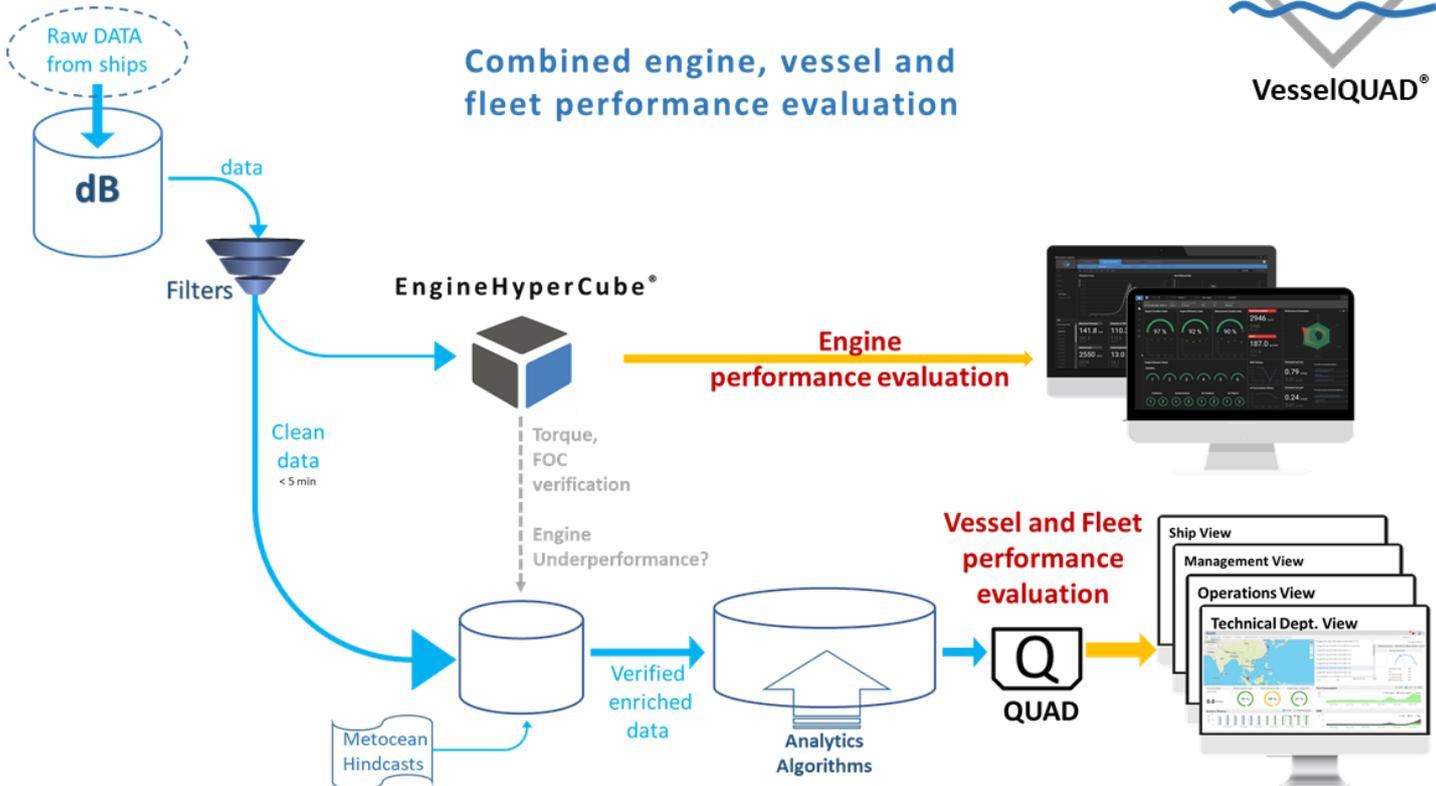
**VesselQUAD®** validates and augments several important but tricky to measure parameters such as Torque, Power, FOC by high fidelity calculated values produced by the propulsion engine digital-twin application **Engine Hyper Cube®**, which also detects any possible engine faults / underperformance.
