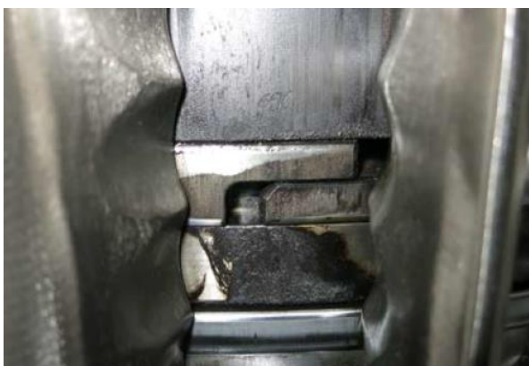
Figure 6: Local scoring/scuffing of 'A' ring gap ends.
