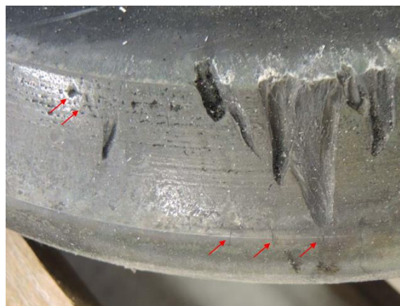
Figure 7: Exhaust valve sealing surface damage.
